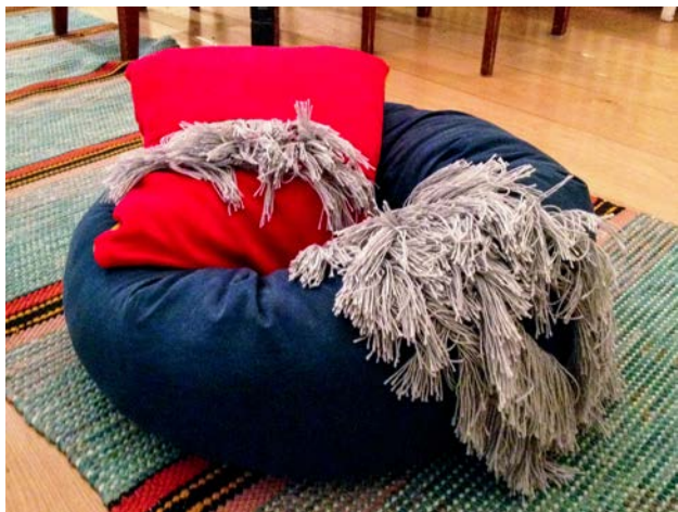
Figure 4. Cushion-shaped musical interface made of conductive yarn.
